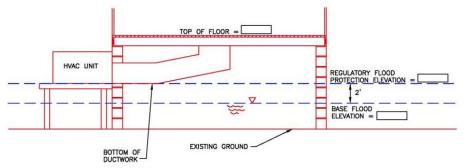
REFERENCE LEVEL IS THE TOP OF THE LOWEST FLOOR OR BOTTOM OF THE LOWEST ATTENDANT UTILITY INCLUDING DUCTWORK, WHICHEVER IS LOWER.
