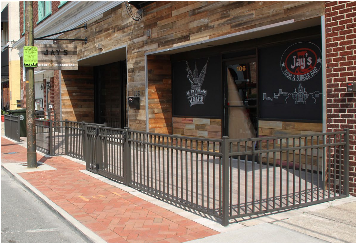
This photograph shows how the dining enclosure moves around a light pole in order to maintain a minimum 5' clearance on the sidewalk.
