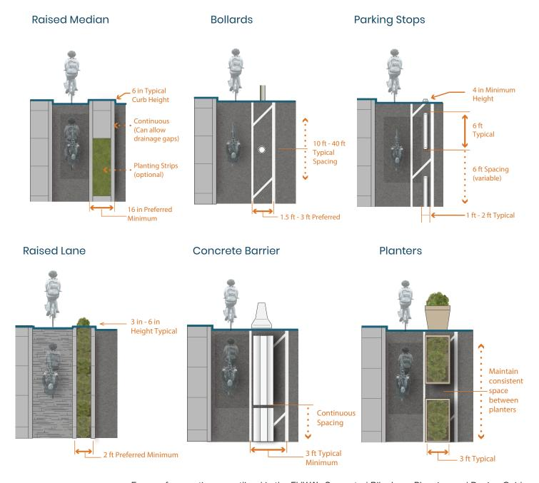
Forms of separation as outlined in the FHWA's Separated Bike Lane Planning and Design Guide.
