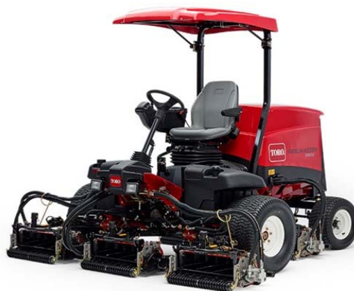
Reelmaster 5510 – used to cut the fairway
