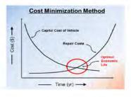
The chart illustrates the annual costs of a vehicle, where the intersection of the capital cost curve with the repair cost curve identifies the point in time where the annual cost of owning the vehicle is lowest (U Curve
